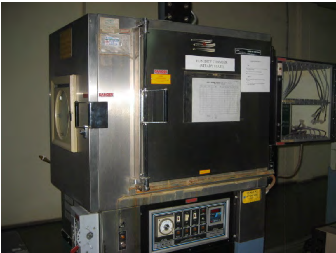
HUMIDITY, STEADY STATE, LOW VOLTAGE TEST CHAMBER (Method 103 as per MIL-STD-202)
