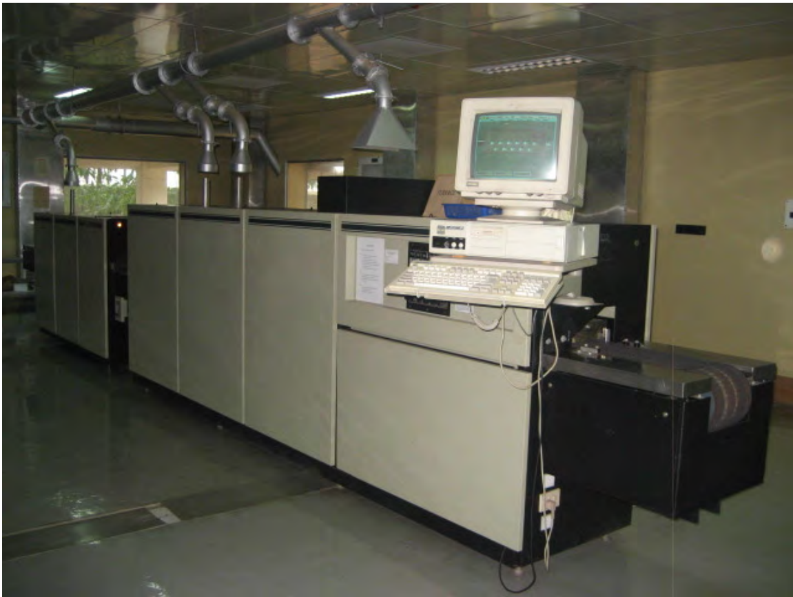
EIGHT ZONE BTU FIRING KILN WITH ATTACHED DRIER
