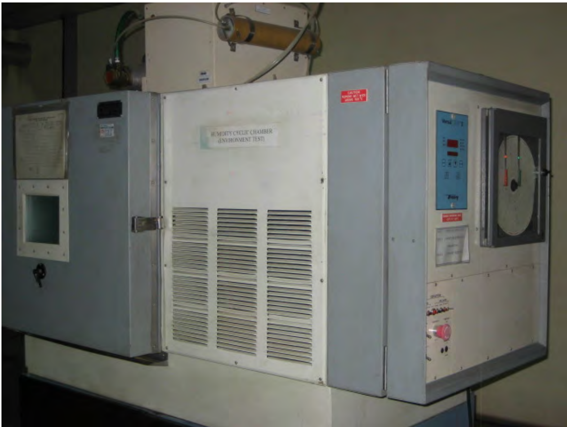
MOISTURE RESISTANCE TEST CHAMBER (Method 106 as per MIL-STD-202)
